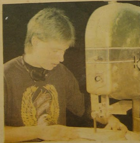
Ryan Faircloth uses a band saw to cut out table lamp parts.
